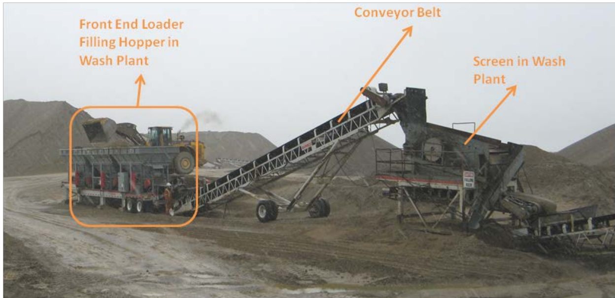
Photo 15: Front End Loader Filling Wash Plant Hopper
